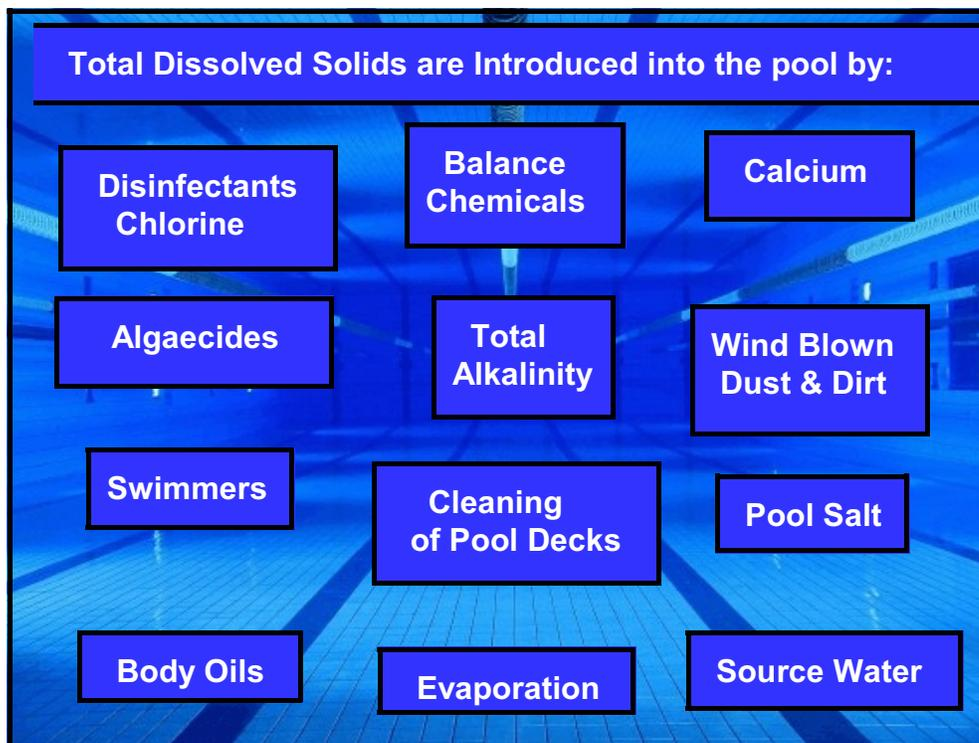
**How do you test for it ?** A TDS Meter measures the TDS level of a water sample by determining the electrical conductivity of the sample. Readings up to 2,000 ppm are common. Over 2,000 ppm we consider high if you are experiencing clarity problems.
